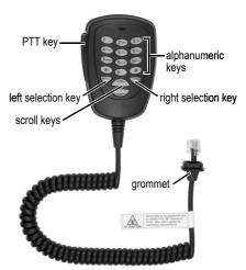
As well as the PTT key, there are twelve alphanumeric keys, two scroll keys, and a left and right selection key on the keypad microphone. The selection keys and scroll keys duplicate the keys on the control head and the 12 alphanumeric keys on the keypad microphone are used to dial call strings and enter text.
